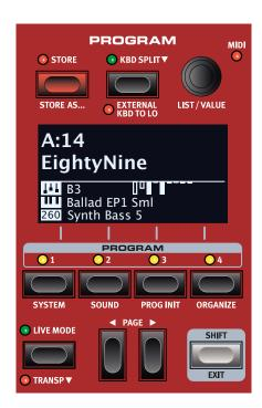
The **PROGRAM** section provides access to performance functions such as loading and storing programs, access to Live programs, keyboard split functionality and more. This is also where menus containing *System* and *Sound* settings are found. The menus and their settings are covered in a separate chapter, starting on page 27.
