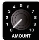
Potentiometer-type *knobs* are used for most panel settings on the Nord Organ 3. When a program is loaded, the physical positions of these knobs will in most cases not correspond to the stored values. As soon as a knob is turned however, its associated parameter value will “snap” to the knob's position.
