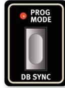
The important **PROG MODE** button determines the behaviour of the LED equipped drawbars. When Prog Mode is lit, *Program Mode* is active and the LED equipped drawbars are using the drawbar settings that belong to the currently loaded program. The setting for each drawbar is in this case indicated with a *single LED*.
