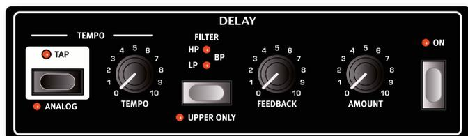
The **FEEDBACK** knob controls the number of delay repeats. At the lowest setting only the initial repeat is heard, while the highest produces a very long feedback tail.
