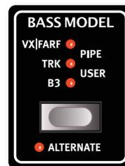
Regardless of selected Organ Model, the Bass Model used for the Bass Pedal registers can be chosen freely among the available options - **B3**, **TRK**, **VX/FARF**, **PIPE** and **USER**. This allows for combining the Upper and Lower manuals of a particular Organ Model with any other Bass Model as desired.
