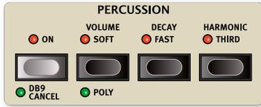
The **PERCUSSION** effect adds extra attack to the sound by having a single envelope generator controlling either the 2nd or 3rd harmonic.
