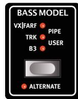
For each of the Organ Models there is a corresponding Bass Model, used for the Pedal Bass drawbars. It is not necessary, however, to pair the Organ Model with its exact counterpart, but Organ and Bass combinations can be chosen freely among the available selections.
