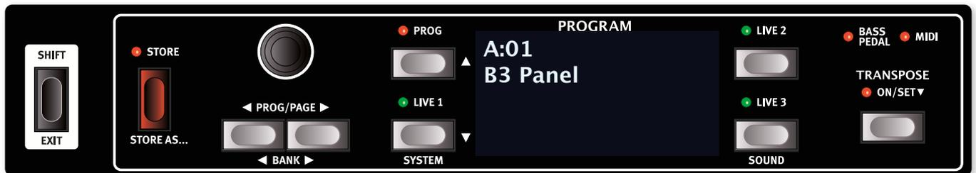
The centrally located **PROGRAM** section provides access to performance functions such as loading and storing programs, access to Live programs, Transpose functionality and more. This is also where menus containing *System* and *Sound* settings are found. The menus and their settings are covered in a separate chapter, starting on page 29.
